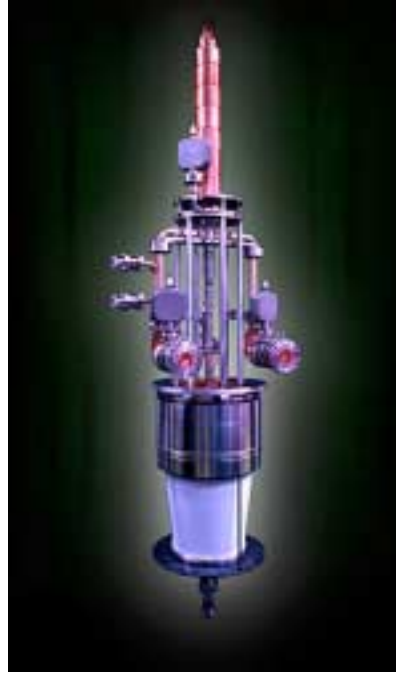
NLC High-Power Klystron
